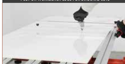
T-CUT ON WORKBENCH EDGE FOR DIAGONAL CUTS
